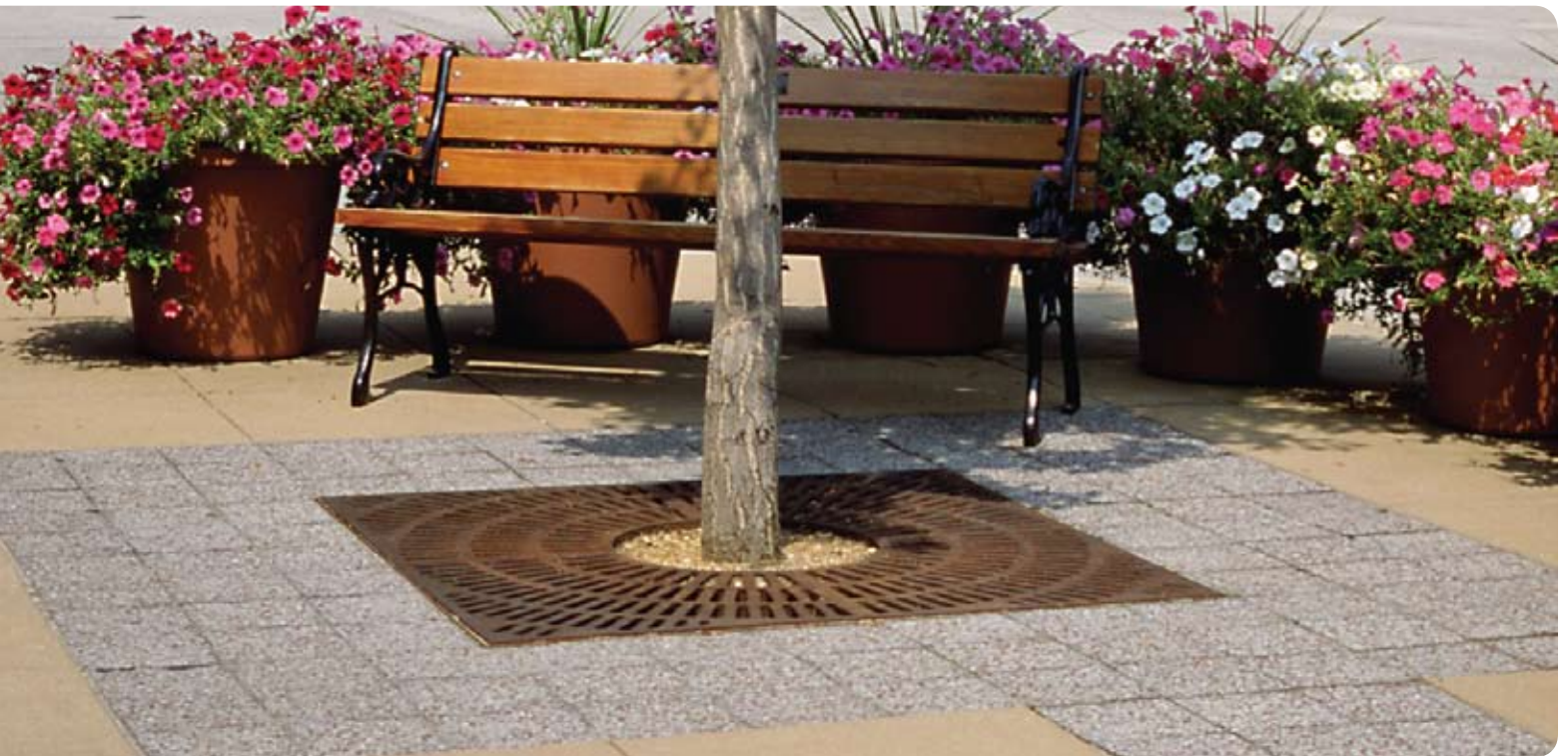
R-8717 • 60" x 60" 36" diameter tree opening. .25" slot openings. 440 pounds per set. (Available with removable insert grate and 16" tree opening, order as R-8717-A . 580 pounds per set.) R-8717 is also a Los Angeles approved grate.
