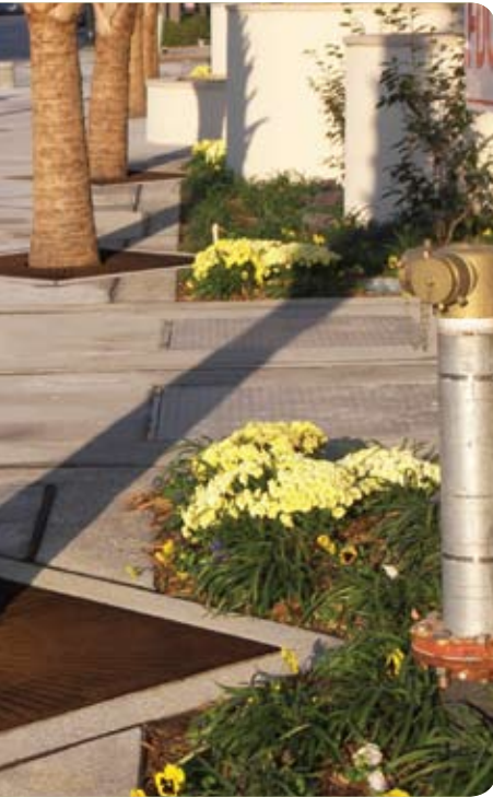
R-8809 • 36" x 72" 18" diameter expandable tree opening. .375" slot openings. 334 pounds per set. (Available as 48" x 72", order as R-8815-1 . 480 pounds per set.) R-8809 is also a Los Angeles approved grate.
