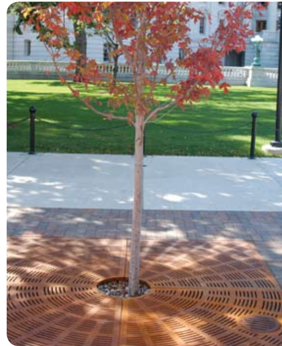
R-8710 • 48" x 48" 12" diameter expandable tree opening. .375" slot openings. Available with cast 16" or 24" diameter tree opening and with light openings. 260 pounds per set. (Also available as 48" round 2-piece grate with 16" diameter expandable tree opening, order as R-8882 . 298 pounds per set.) R-8710 is also a Los Angeles approved grate.
